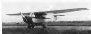
WINGS EXTENDED , Bryon roadable starts takeoff. Costing $250, plane took 15 hours to build. It was easily salvaged from a plane; tail and engine are from a Cessna Ruby A-6.
